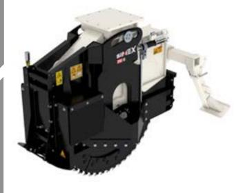
Intended for excavator boom mounting, they are specially indicated for cutting and narrow trenching for fiber optics installation on hard and compact surfaces: asphalt, concrete and rock. Slides parallel to the ground. Constant trenching depth. Mechanical or hydraulic adjustment of trench depth. Disk with removable, interchangeable segments allows quick variation of the trench width while maintaining the same base wheel. (RWE 50).
